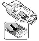
**Note:** When you need to remove the SIM card, slide it, as shown, and take it out of the socket.
