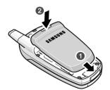
**5.** Press the battery down until it clicks into place. Make sure that the battery is properly installed before switching on the phone.
