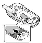
4. Place the battery so that the tabs on the end align with the slots at the bottom of the phone.
