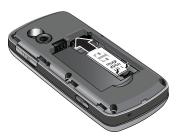
Note: If the card is not inserted correctly, the phone does not detect the SIM card. Remove the battery and re-orient the card back into the slot.
