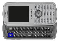
When you slide the phone open, the display rotates from a vertical viewing mode to a horizontal viewing mode.
