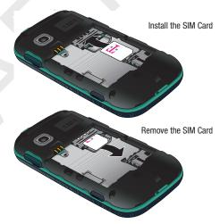
Carefully slide the SIM card into the SIM card socket until the card is secured into place. Make sure that the card's gold contacts face down and that the upper-left angled corner of the card is positioned as shown.
