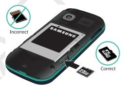
Firmly press the card into the slot and make sure that it catches with the push-click insertion.
