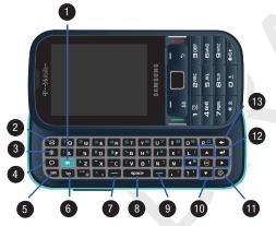
Using the QWERTY keyboard, you can type letters, numbers, punctuation, and other special characters into text entry fields or other applications simpler and faster than using the telephone keypad.
