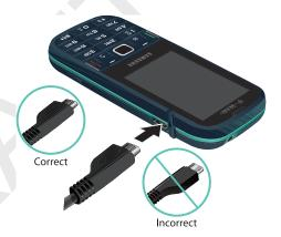
Note: This illustration displays both the correct and incorrect orientation for connecting the charger. If the charger is incorrectly connected, damage to the accessory port will occur therefore voiding the phone's warranty. 4. When charging is finished, first unplug the charger's power plug from the AC wall outlet, then disconnect the charger's connector from the phone.
