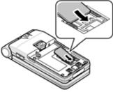
4. To remove the SIM card, slide it upwards as shown.
