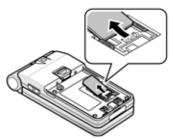
5. Replace the battery so that the tabs on the end align with the slots at the bottom of the phone.
