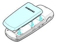
6. Press the battery until it clicks into place. Make sure that the battery is properly installed before switching the phone on.
