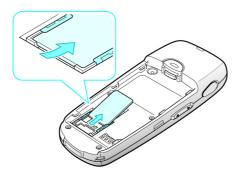
5. Place the battery so that the tabs on the end align with the slots at the bottom of the phone.
