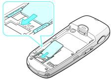
Note: When you need to remove the SIM card, slide it, as shown, and take it out of the socket.
