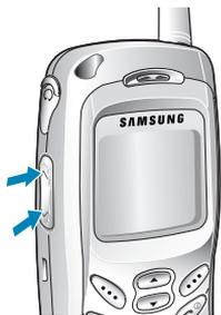
In standby mode, you can adjust the key beep volume using these keys.
