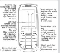
Press and hold up in Idle mode to activate or deactivate the SSR SSR mode (Simple Smart Ringtone) mode. The SSR mode is for alerting you to incoming calls in noisy places, by simultaneously vibrating and
