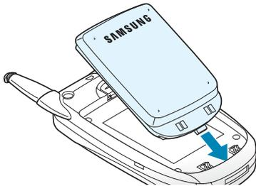
2. Press the battery down until it snaps into place. Make sure that the battery is correctly installed before switching on the power.
