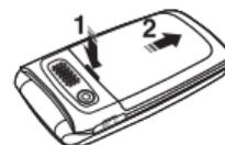
2. Unlock the microSD card slot by carefully sliding it up. The metal cover should now easily lift up.
