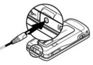
You also may charge the battery with a USB cable with power from a computer.
