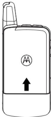
2. Remove the battery cover from the back of the phone
