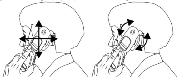
If your HA has a telecoil, activate its switch, then also rotate the handset as illustrated to align the telecoils.
