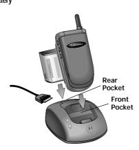
**Note:** If two batteries are loaded in the charging base, the batteries will charge one at a time, the front pocket first, followed by the rear pocket.
