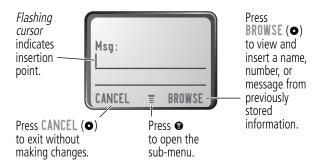
When you enter text, the flashing cursor changes to a *block cursor*, and the soft key functions change:
