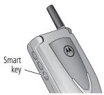
For example, if you highlight an item and press the smart key, the smart key selects the highlighted item. You can use the smart key to send and end calls, select menu items, toggle features on and off, and open your phonebook. The smart key usually performs the same function as the right soft key ( $\bullet$ ).
