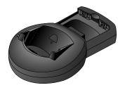
This charging base can be loaded with up to three batteries. Equipped with one LED charging status indicator for each battery, the charging base's front pocket can charge both a main and an auxiliary battery attached to a phone, and the rear pocket can charge one battery by itself. For use with Lithium Ion, Nickel Cadmium and Nickel Metal Hydride batteries.
