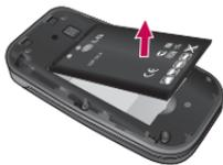
**Warning!** Do not remove the battery when the phone is turned on; this can damage the phone.
