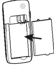
You must install and charge the battery to use your phone. Insert the ridge at the side of the battery into the base of the phone, then push the battery down and snap it into place.
