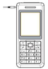
Step 2: Connect the charger to the phone. Plug the charger into a power socket. The charger connection screen will be displayed.
