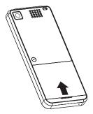
Step 1: Flip the battery cover up to remove it.
