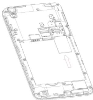
3. Insert the memory card into the card slot with the metal contacts facing down until it inserts to the right position.
