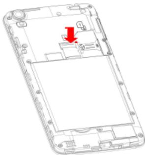
4. Insert the battery by aligning the gold contacts on the battery with the gold contacts in the battery compartment. Gently push down on the battery until it clicks into place.
