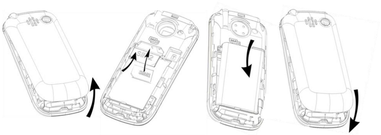
Likewise, to remove the SIM card, switch off the phone, remove the battery and then take out the SIM card.
