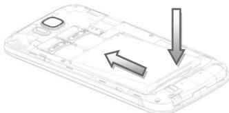
For the battery cover, fix the top hooks of the back panel to the phone body and press the battery cover on to the phone, as shown above.
