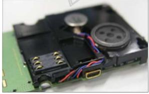
• Detached antenna and main board (while installing the antenna, make sure the antenna contact blade well contacted with the contacts)
