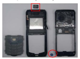
• Be careful with the correct installation of motor and speaker and the winding positio
