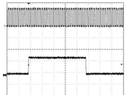
32 R1238 (Lower) SIMCLK (Accessing SIM after power-on) C1236 (Lower) SIMDAT (Accessing SIM after power-on) (CH1, CH2=2V, 2μs/div)
