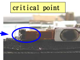
< 3. Check FPCB attachment >
