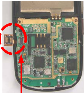
&lt; Close the Key-FPCB Connector &gt;
