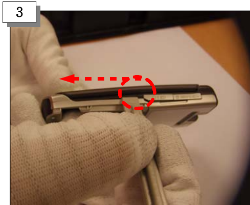
Disjoint the Hooks of REAR
