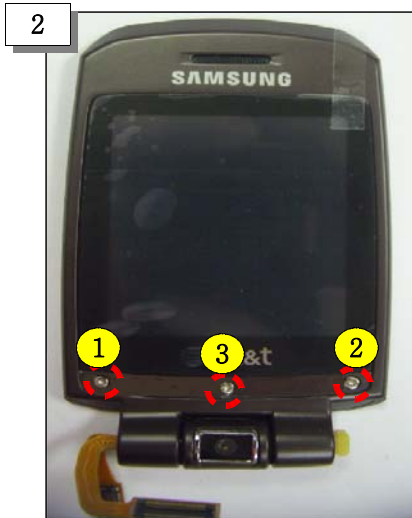
Tighten the SCREWS(3 points)
