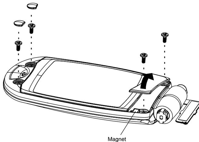
3. Separate the upper cover and upper case using a plastic strip (of credit card thickness).
