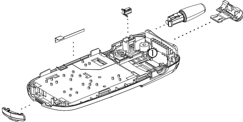
4. Place the headset jack cover in the lower case cover. Assemble the lower case with the lower cover assembly. Close the four snaps making sure that both assemblies are connected.
