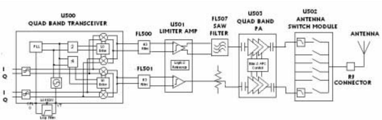
Figure 4.3: Transmitter Block Diagram
