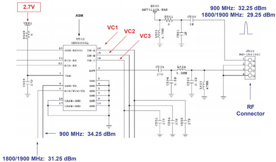
Figure 8.6: Front-end Module (U502), transmit-path signals
