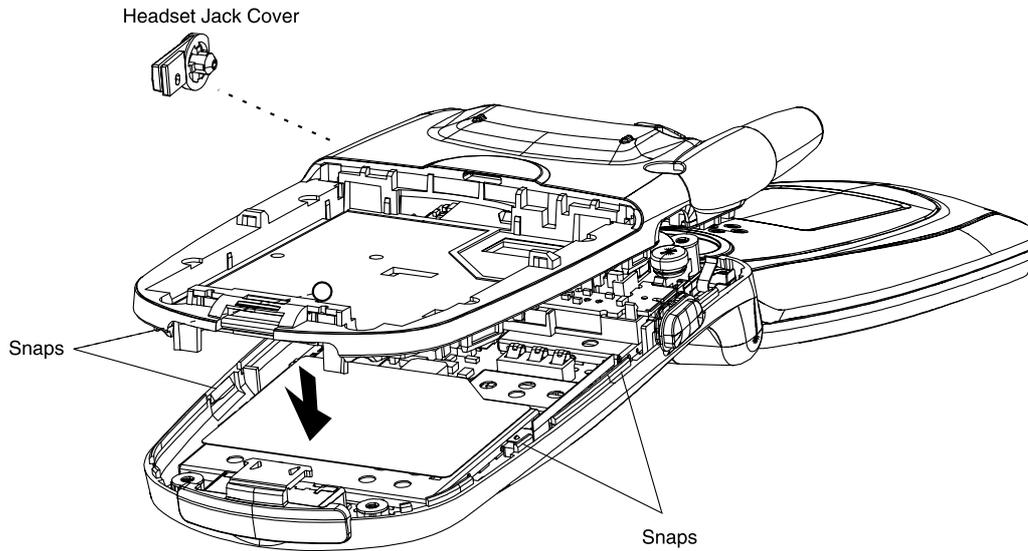
5. Insert four screws and torque all screws to 1.3 KGF-CM using a #3ULR0 Trident screwdriver tip. Replace the two screw caps.
