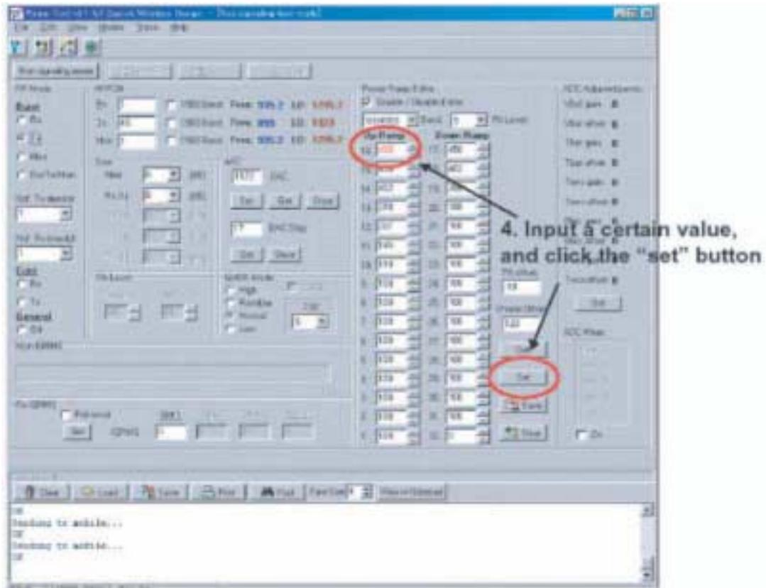
5. Repeat Step 4 (input and set) until the target power level is displayed on the power meter. (Refer to the **Calibration Specification** tables at the end of this section for target power levels.)
