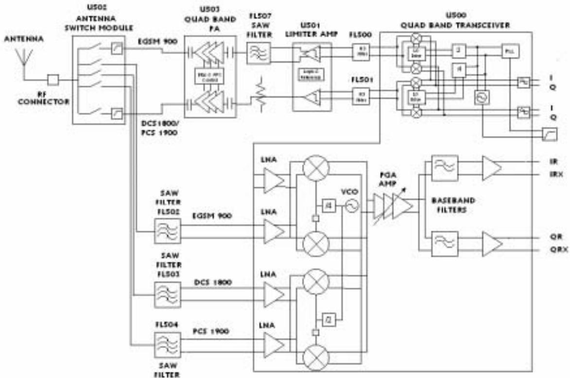
Figure 4.1: RF Block Diagram
