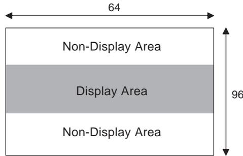
Figure 4.9: Sub-LCD Dimensions
