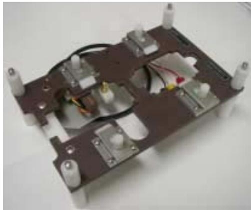
Figure 5.1: PCB Repair Jig
