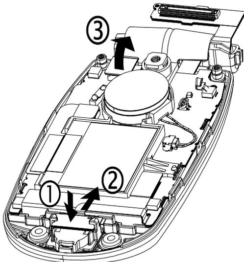
5. Lift bottom end of flex PCB board and slide right until board clears the camera and is free from the upper cover. The hinge pivot will exit the hinge compartment while removing the flex PCB board.
