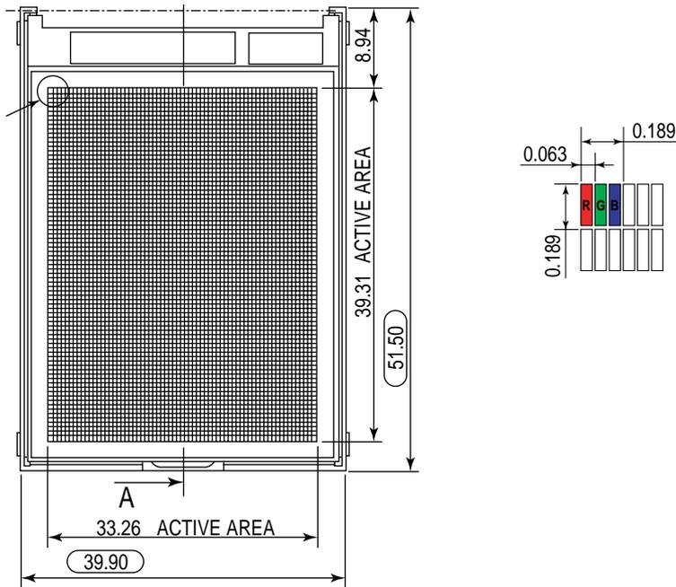
**Figure 4.7: Main LCD Dimensions**
