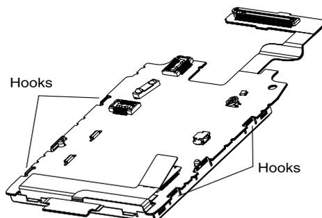
4. Remove main LCD module.
