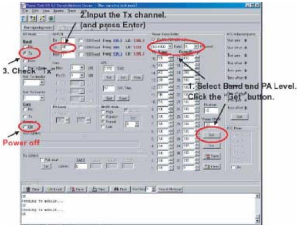
To adjust the DAC to obtain the desired Tx power level:
