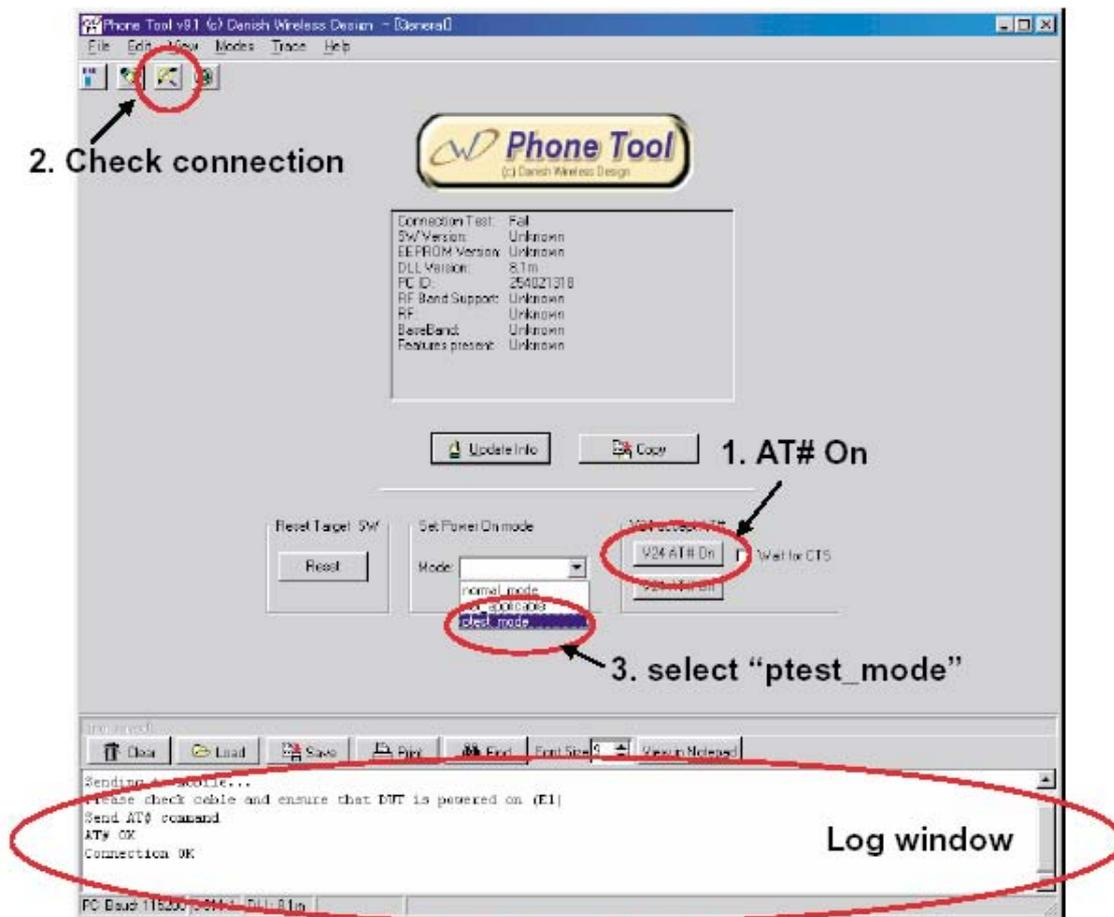
1. Click the "V24 AT# On", and check the log window. >>> "AT# OK"
