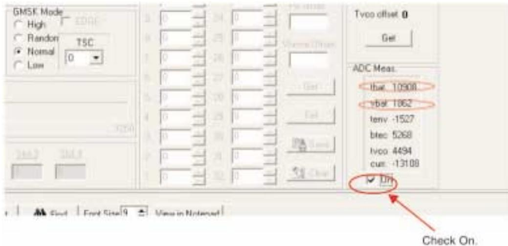
3. Check the "On" box located on the bottom of the ADC Meas(urement) box.
