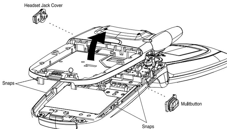
7. Using the edge of a plastic strip (of credit card thickness) carefully separate the connector from the case. Remove the Main by lifting the bottom end up first, then gently twisting (pivot) until the PCB separates from the 80 pin connector. If the Main PCB is connected to the 80 pin connector, carefully use edge of plastic strip (of credit card thickness) to separate.
