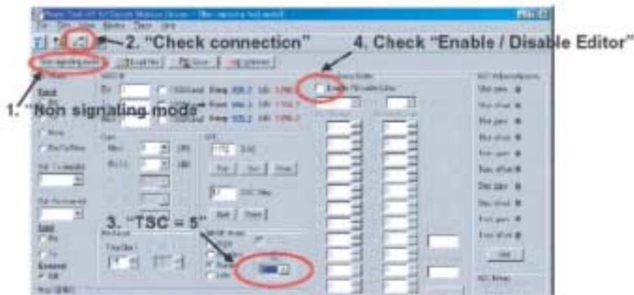
To begin calibration of the transmitter, select **"Non-Signaling Test"** from the **"Modes"** pull-down menu in PhoneTool and complete the following steps:
