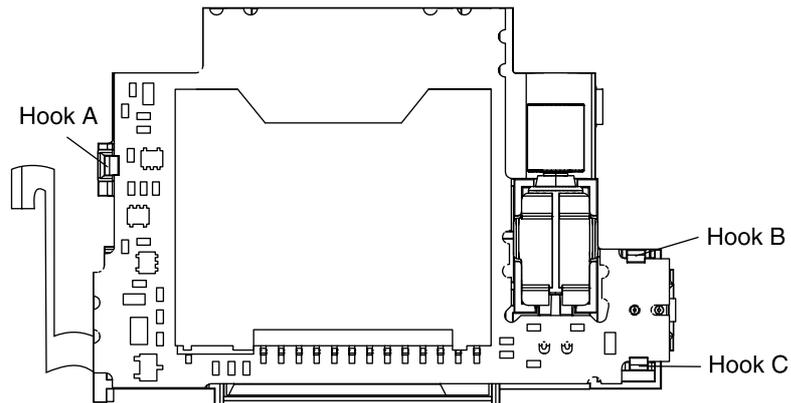
4. Pivot (1), lift (2) and remove sub PCB.
