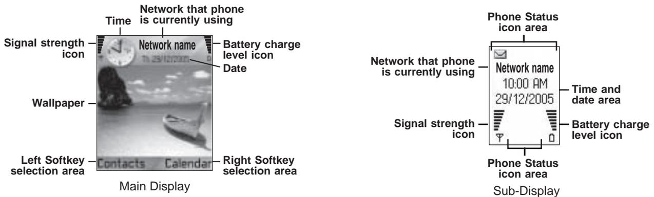
Figure 3.3: Main & Sub Liquid Crystal Displays
