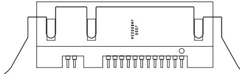
External I/O connector is a 14-pin user interface connector that provides external UART, USB, charger and other interface to the X700 handset.
