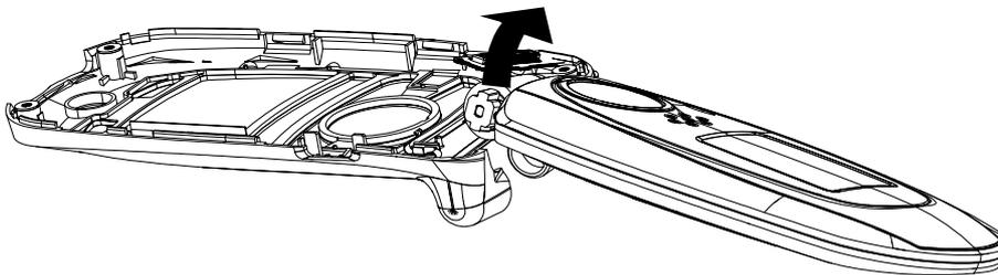
2. Using a strip of plastic (of credit card thickness) gently lift up and remove the logo panel. Remove the two screw caps. Use a Trident screwdriver to remove the four screws securing the logo panel. Retain the screws for reassembly.
