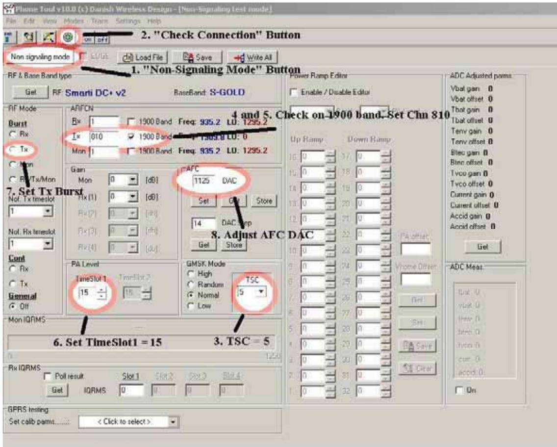
To begin calibration of the VCTCXO, select "Non-Signaling Test" from the "Modes" pull-down menu in PhoneTool and complete the following steps:
