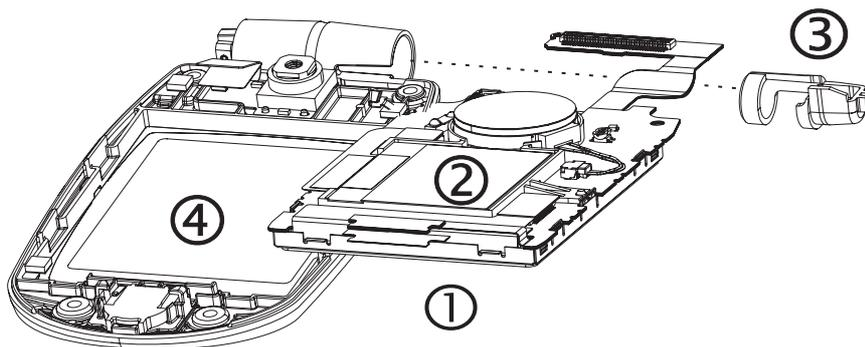
4. Attach the PCB connector into the receiver (1) and (2).
