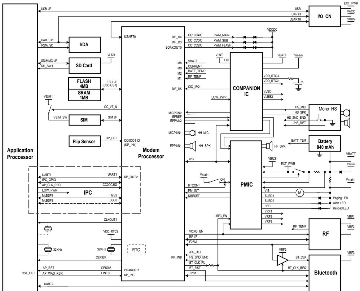
Figure 4.5: Baseband Block Diagram
