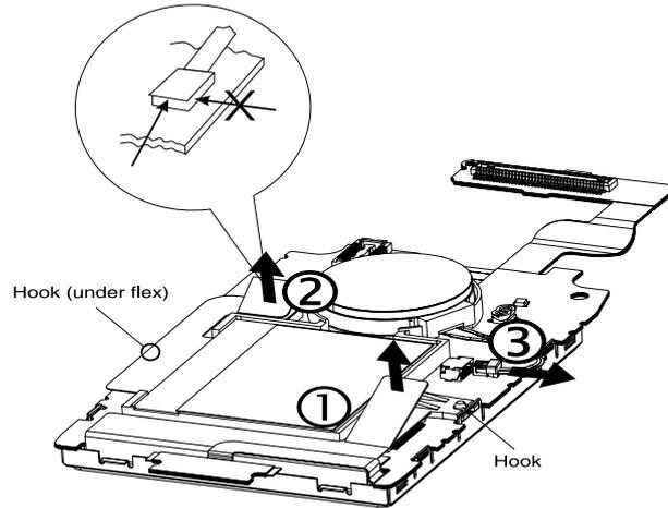
2. Lift and remove sub LCD module.
