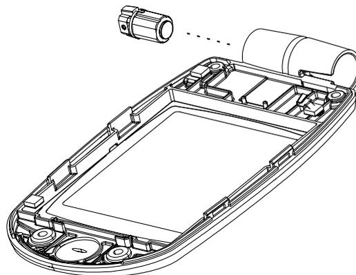
2. 1) Rotate and align the hinge pivot with the open area facing upward and carefully insert into the main area of the lower cover assembly, taking care to tilt the upper housing assembly without causing damage to the flex circuit during reassembly. 2) Push down gently until the upper housing assembly is full engaged into the lower cover. Insert microphone.
