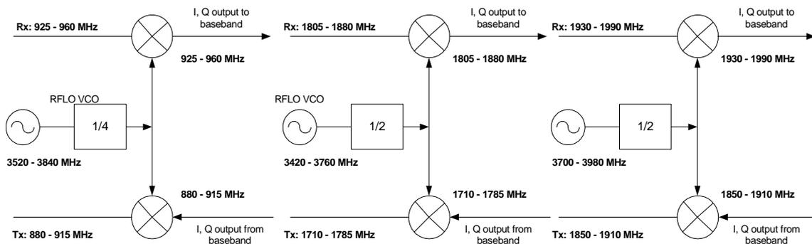
Figure 4.2: Frequency Plan
