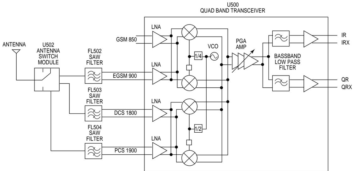
**Figure 4.4: Receiver Block Diagram**
