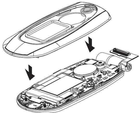
2. Locate the four screws and torque to 1.3 KGF-CM using a #3ULR0 Trident screwdriver tip.
