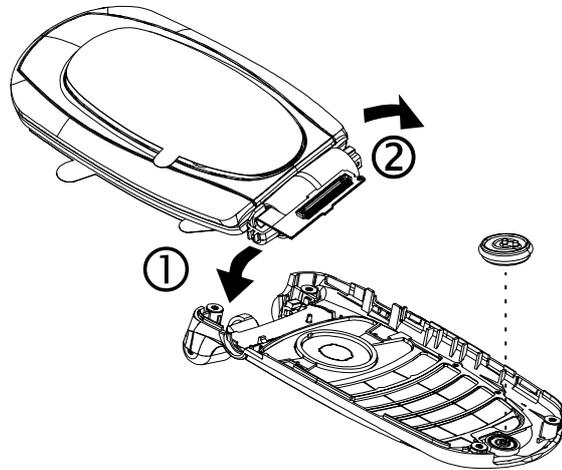
3. 1) Insert hinge holder into the lower cover in the direction shown. 2) Gently lower the other side of the hinge holder into the lower cover. Insert the retaining screw and torque to 1.3 KGF-CM using a #3ULR0 Trident screwdriver tip.
