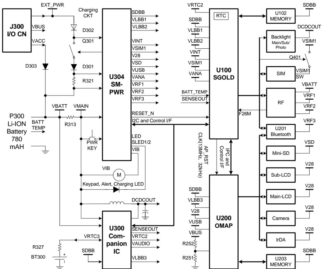
Figure 4.11: Power Supply and Related Sub-System Block Diagram
