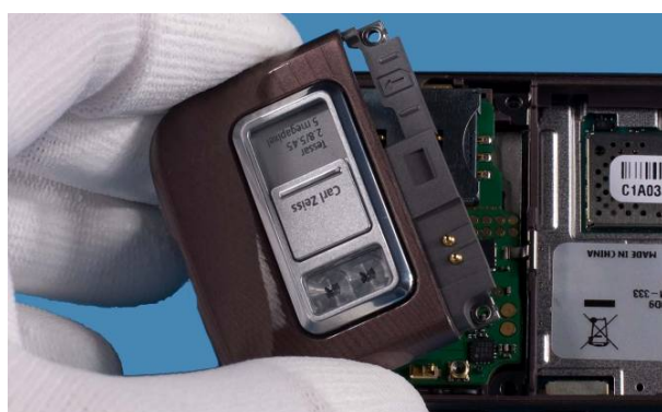
4) After releasing the screws remove the BACK COVER .
