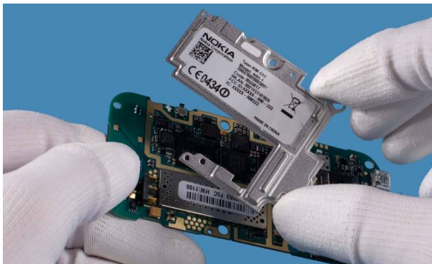
15) Separate the BB SHIELD from PWB .
