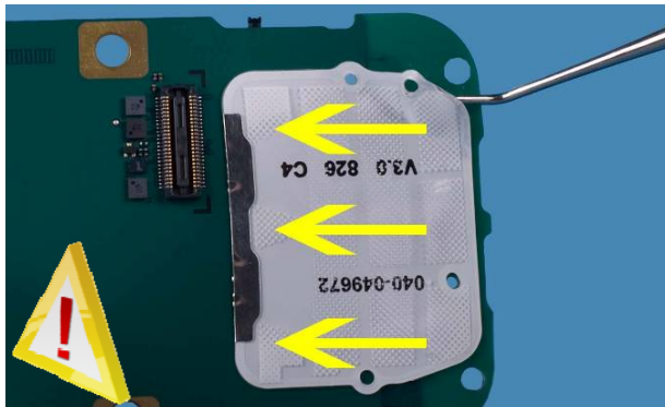
19) Release the DOMESHEET with a dental pick.
