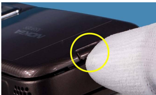
1) Push button and unlock the BATTERY COVER .
