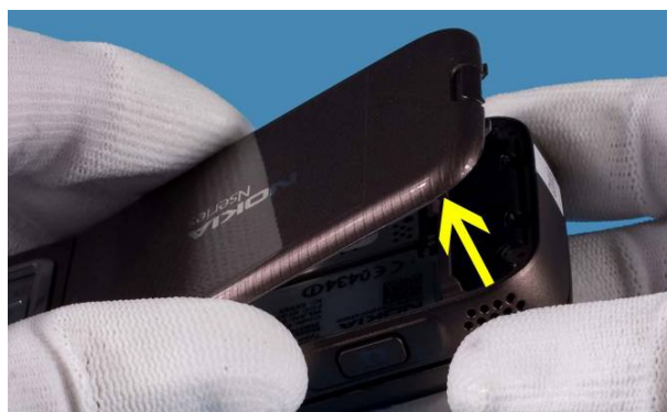
2) Lift up and remove the BATTERY COVER .
