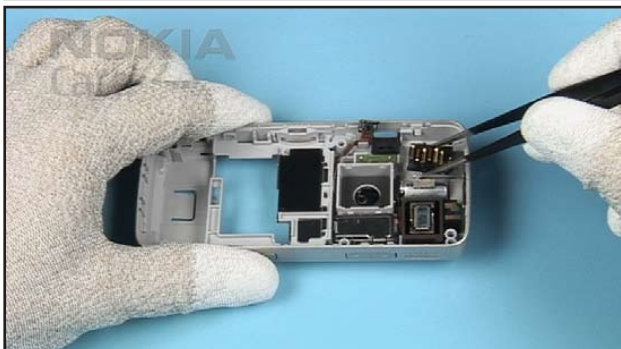
15. Place the AUDIO CONNECTOR into the B-COVER...
