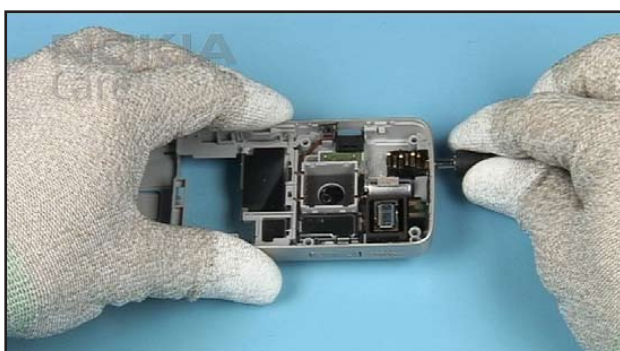
35. Use a 3.5mm headset plug to unlock the AUDIO CONNECTOR.
