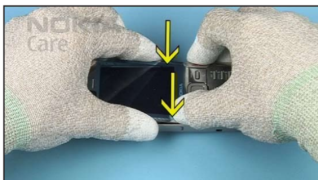
43. Fit the WINDOW ASSY starting at the shown side.
