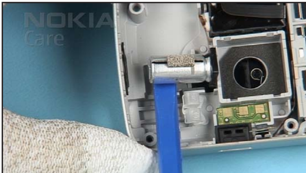
41. Carefully remove the CAPACITOR with the SS-93.
