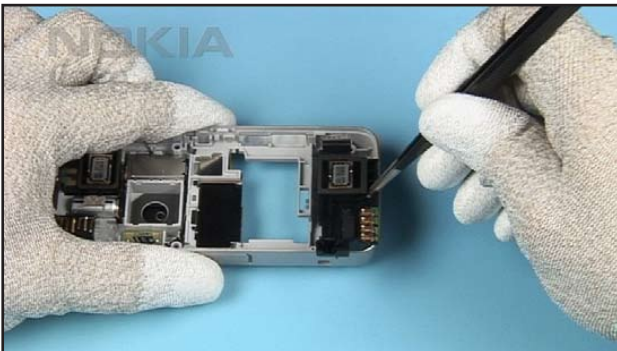
17. Place the ANTENNA CELLULAR ASSY into the B-COVER.
