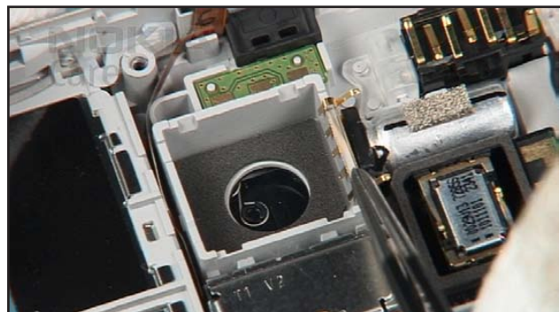
20. Carefully fit the CAMERA GROUNDING SPRINGS.
