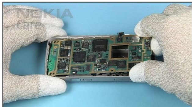
24. Carefully place the ENGINE MODULE onto the B-COVER.
