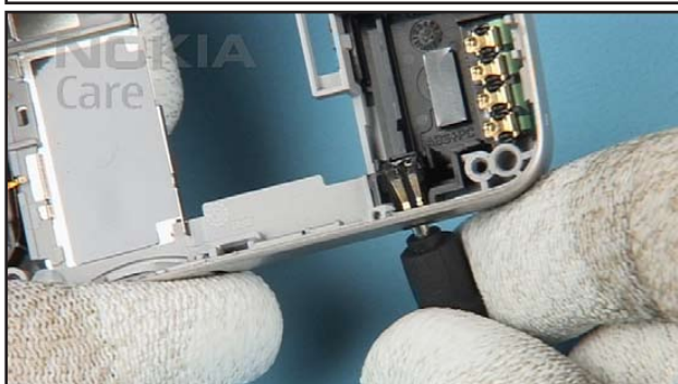
31. Remove the DC-JACK with the DC-Plug.
