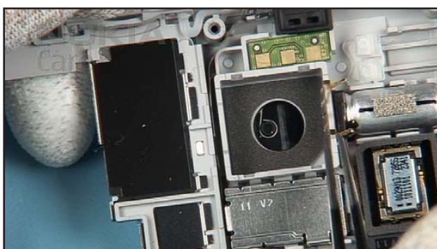
37. Carefully remove the CAMERA GROUNDING SPRINGS.
