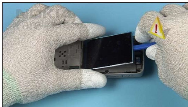
18. Very carefully lift the LCD from the MAIN FRAME.
