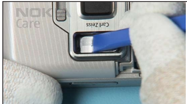
42. Remove the FLASH from B-COVER.
