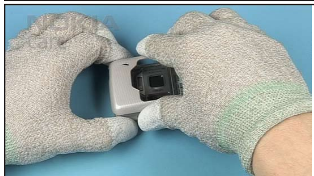
48. Move the D-COVER a bit to the left and remove it.
