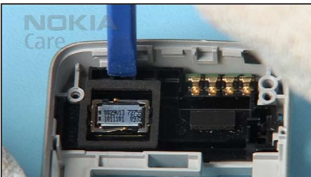
19. Press the other side of the ANTENNA into place.
