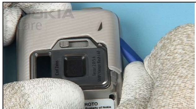
46. Gently unlock the D-COVER ASSY with the SS-93.
