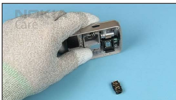
36. AUDIO CONNECTOR drops out by turning the B-COVER.
