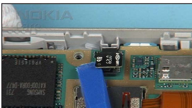
27. Carefully open the FLASH MODULE CONNECTOR.
