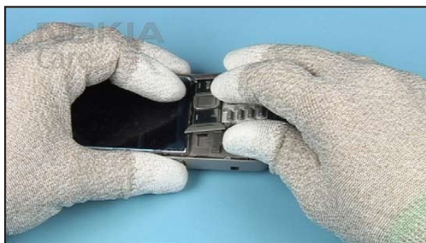
14. Turn the UI MODULE to the shown side..
