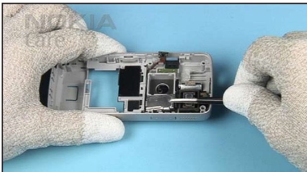
13. Place the FLASH HOLDER onto the FLASH...
