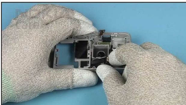
43. Carefully remove the FLASH MODULE...
