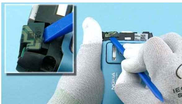
25) Release the COMBO ANTENNA with the SS-93.
