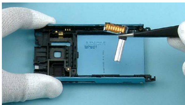
49) Remove the FLASH MODULE with the tweezers.
