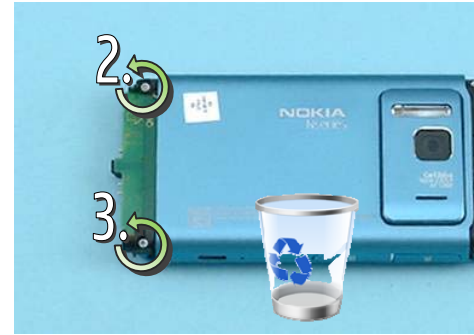
14) Unscrew the four Torx+ size 5 screws order shown. These screws cannot be used. Discard them.
