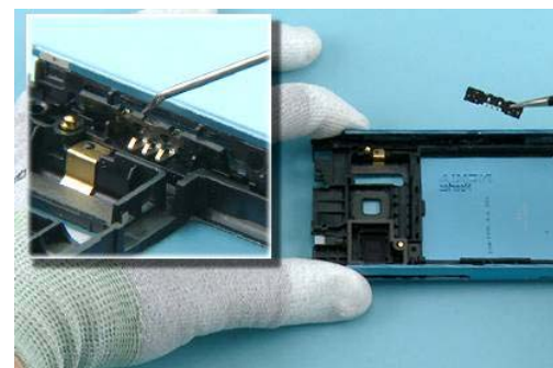
50) Release the SIDE SWITCH with the dental pick. Remove it with the tweezers.
