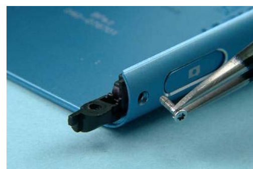
54) Remove the screw with the tweezers.
