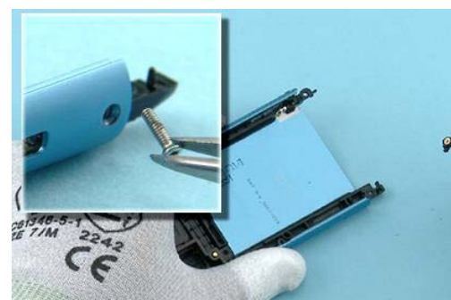
52) Remove the screw and the FIXING NUT with the tweezers.
