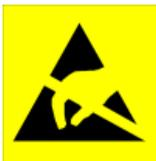
Electrostatic discharge can easily damage the sensitive components of electronic products. Therefore, every Service Supplier must observe the precautions, mentioned in the appropriate "Service Partner Requirements", available on NOKIA Online. Also see ESD Protection Requirements in this Service Manual.
