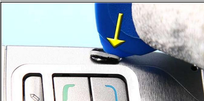
39. Remove the SCREW CAPS with the SRT-6. Note: Do not reuse the SCREW CAPS.
