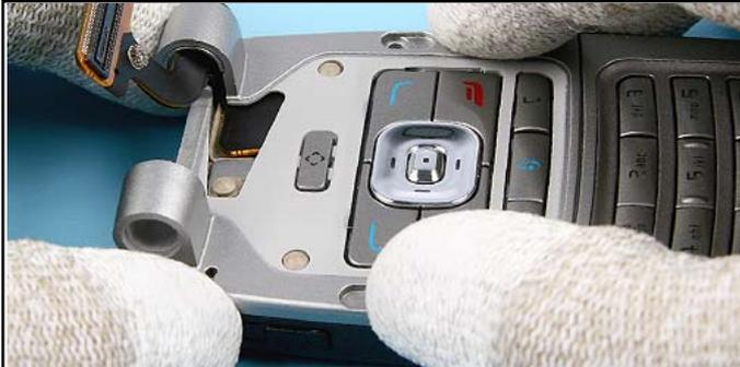
25. Fit the C-COVER into the D-COVER and check the correct position of the FLEX.
