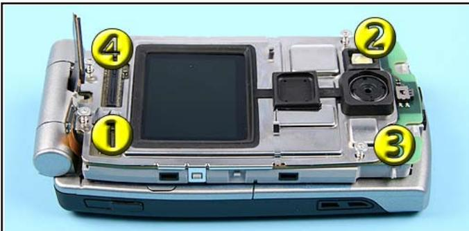
47. To prevent damaging the plastic threads, turn the screws slightly left first. Then tighten them in the shown order with a torque setting of 17Ncm.
