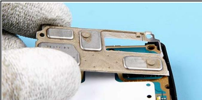
45. Remove the SHIELD KEY.
