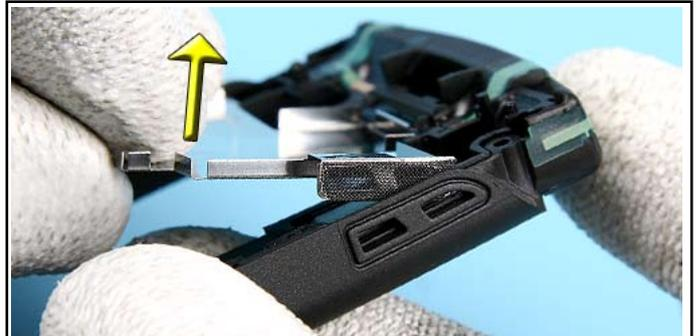
58. ...and lift it from the D-Cover. Do not bend the IHF SHIELD.
