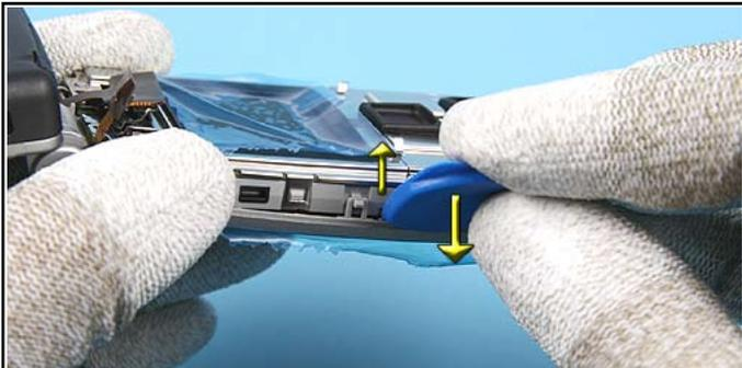
13. Open the unit and unlock the snap of the B-COVER ASSY.
