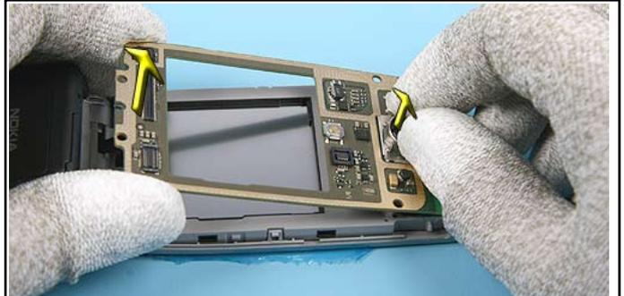
18. Lift the LR LID PWB and the CAMERA as shown and remove the modules carefully.
