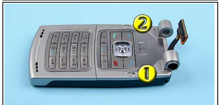
40. Unscrew the two, Torx Plus® size 5 SCREWS in the order shown.
