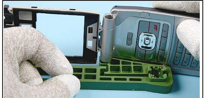
34. Use the SS-15 as a support when removing the HINGE. Position the HINGE exactly over the recess.
