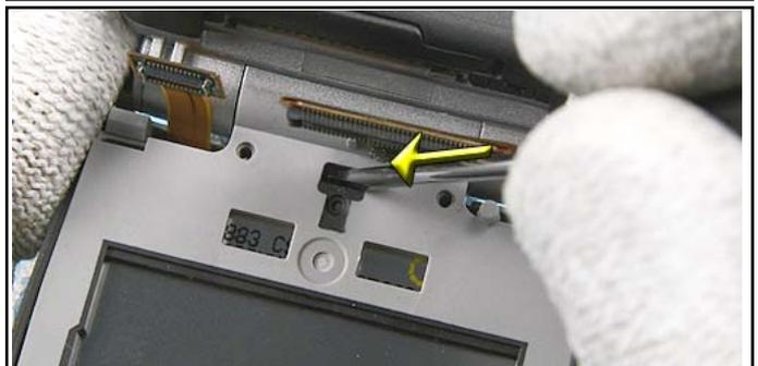
24. Then, release the snap in the middle of the cover with a slotted screwdriver.
