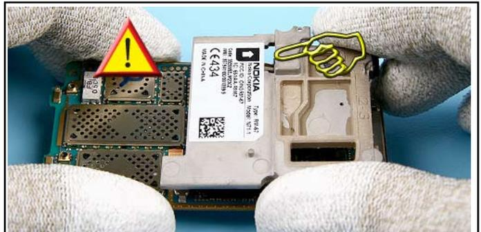
62. Remove the CENTER SHIELD paying attention to the Battery Connector.
