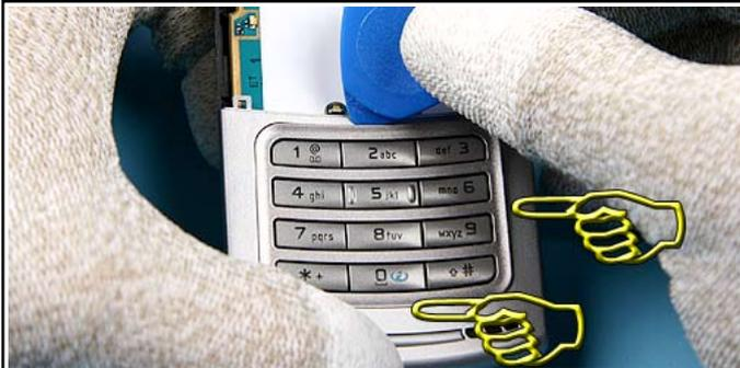
49. Fit the SRT-6 between the C-COVER SLIDE SURROUND and the C-COVER and unlock the C-COVER SLIDE SURROUND.
