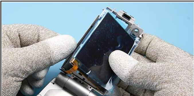
29. Protect the LCD with a film and remove it from the LID CENTER FRAME.
