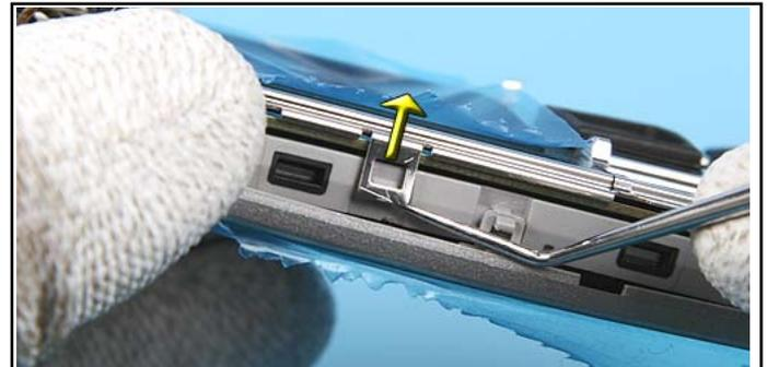
14. Then unlock the SHIELD LID ASSY by using a dental tool. Do the same on both sides.
