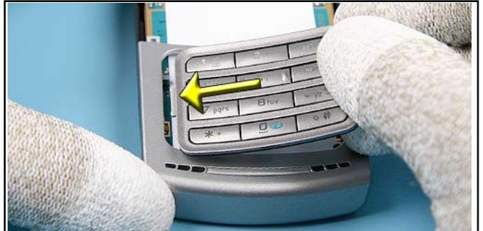
18. Insert the KEYMAT assembly as shown.
