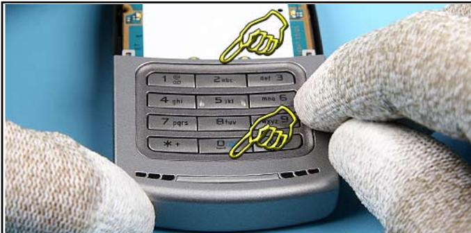
19. Secure the KEYMAT assembly by pressing it into place.
