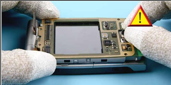
41. Place the LR LID PWB onto the LID CENTER FRAME and check the position of the CAMERA MAIN ASSY.
