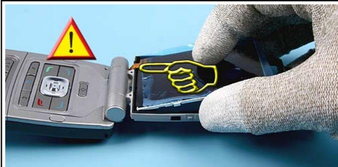
37. Place the LCD onto the LID CENTER FRAME.
