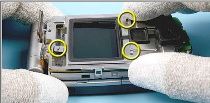
45. Fit the SHIELD LID ASSY into the LID CENTER FRAME. Take special care to the grounding springs.
