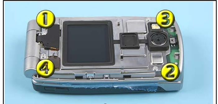
10. Unscrew the four, Torx Plus® size 5 SCREWS in the order shown.
