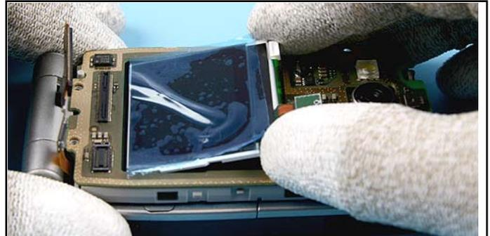
42. Fit the LCD into its place.
