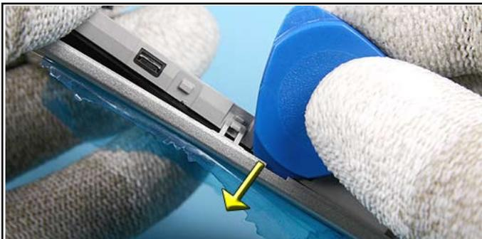
27. Place the SRT-6 between the B-COVER and the LID CENTER FRAME and release the last two snaps.
