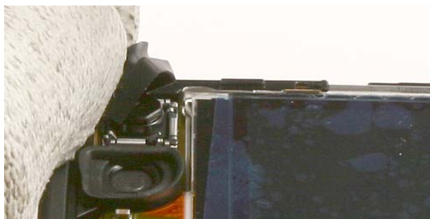
12.) Remove the Camera gasket .
