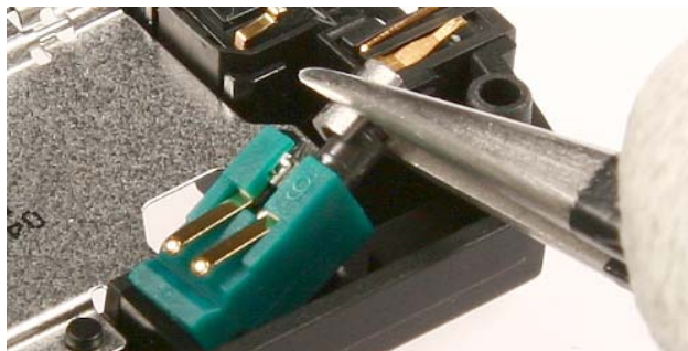
26.) Remove the Vibra Motor with tweezers.
