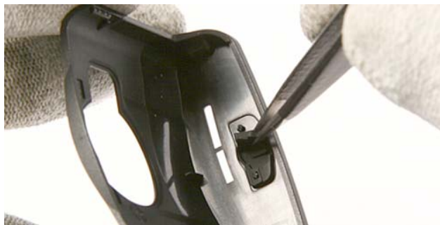
10.) Remove the Power Button with tweezers.
