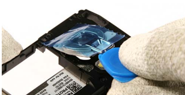
32.) Lever out the Camera Rear Bezel Assy .
