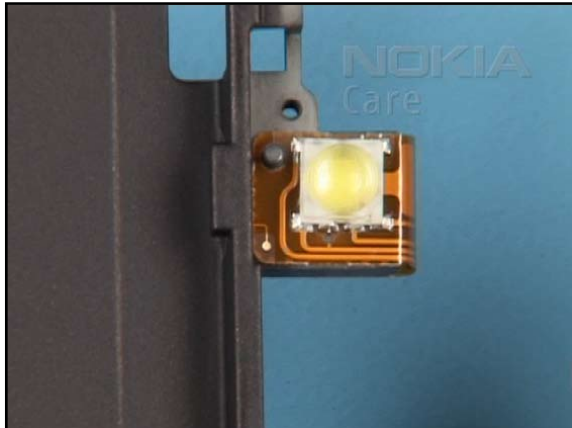
2. Note that the FLASH MODULE is very delicate and becomes useless in consequence of mechanical stress.
