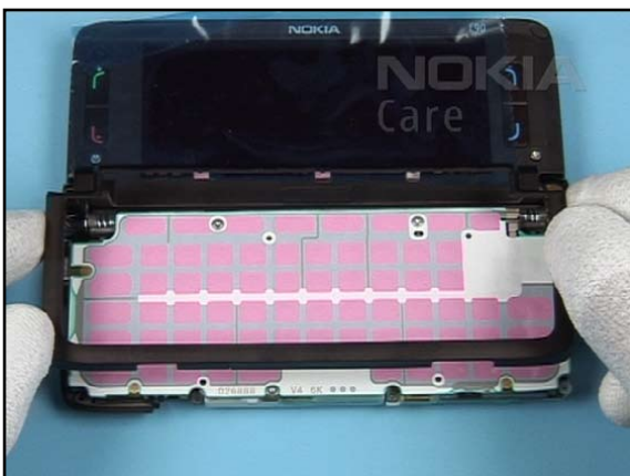
23. Replace the QWERTY COVER, beginning on the left side, where the connectors are located.
