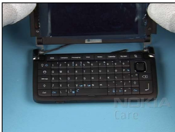
3. Fit the C-COVER. Note the correct alignment to the mounting parts of the hinge.
