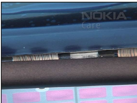
24. Close the clips, check that no cables will be squeezed, otherwise the DUAL AXIS HINGE MODULE becomes unusable.
