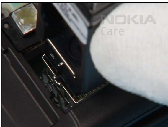
29. Mind the alignment tab while replacing the CAMERA MODULE.
