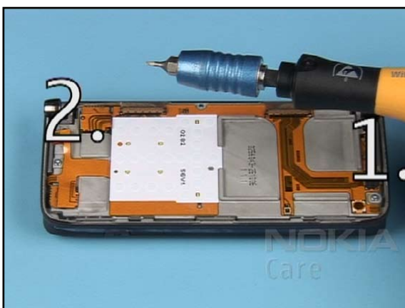
12. Unscrew these 2 Torx Plus size 4 screws.
