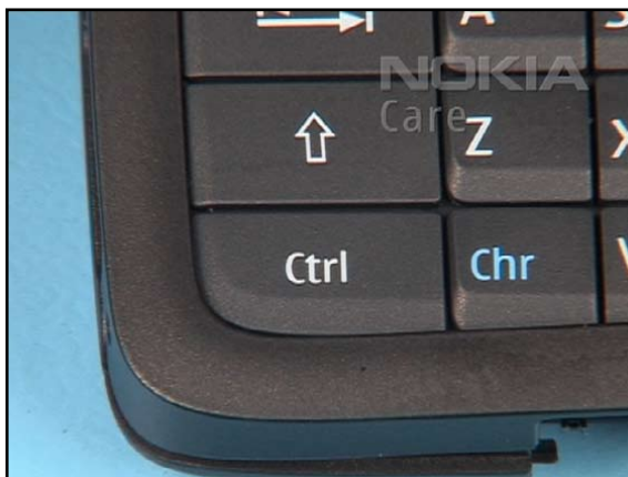
20. Mind the correct positioning of the key mat before going on.
