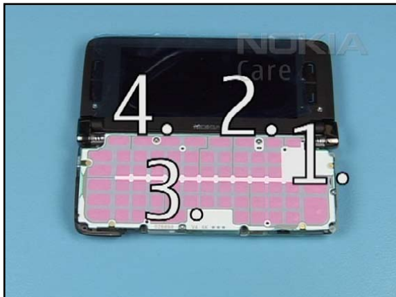
20. Unscrew these 4 Torx Plus size 4 screws in the order shown.
