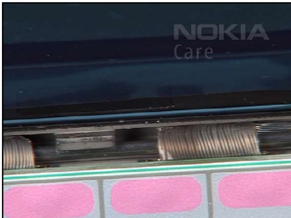
18. Check the correct placement of the cables before going on.
