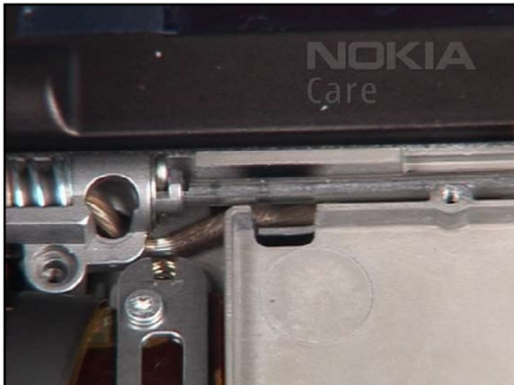
10. Note: False placement will destroy the delicate MICROCOAX cables.
