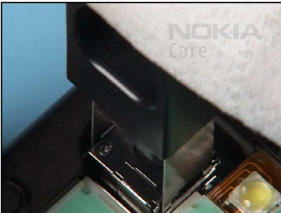
9. Gently push it down. The clips of the housing are released now.
