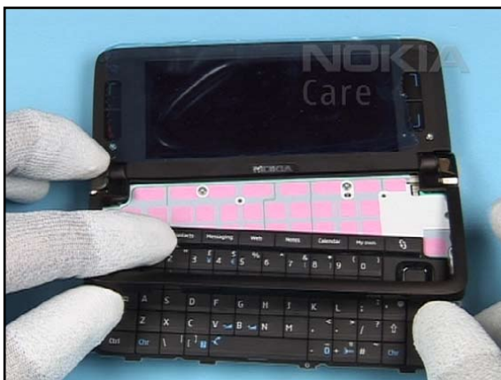
16. It is possible to remove the QWERTY KEYMAT without unlocking the QWERTY COVER.
