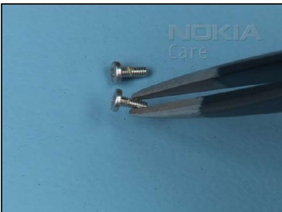
11. Insert the 2 hinge screws. Note! Use the correct length - M1.4 x 4.5
