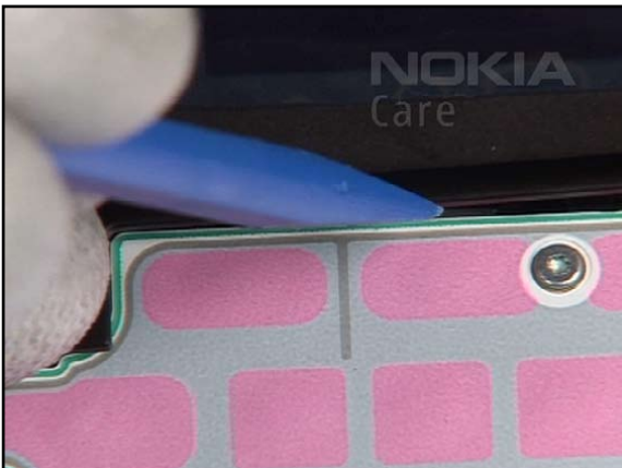
19. ...and on the left side near the hinge. After that, the QWERTY COVER can be removed easily.
