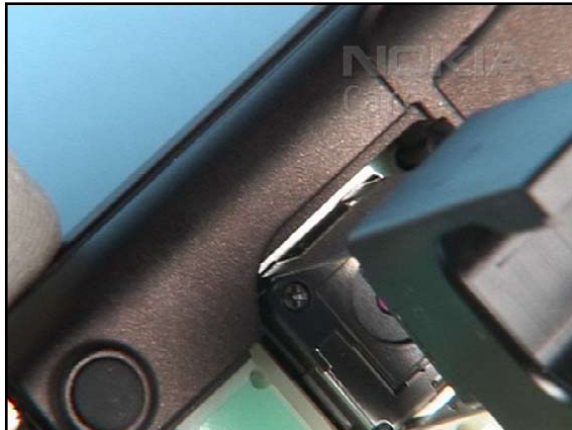
8. Insert the SS-81 into the housing of the CAMERA MODULE. Note the correct positioning of the tool.
