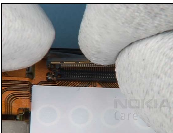
6. Close both MICROCOAX HARNESS connector. Check for correct fitting of the connectors before going on.
