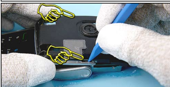
16. The FLIP MODULE is attached to the B-COVER with two snaps.
