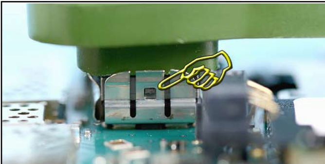
43. Press the SS-15 lightly in shown direction until the CAMERA MODULE have been unlocked.
