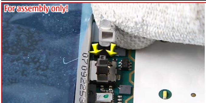
13. Note the correct position when reassembling the JOYSTICK.
