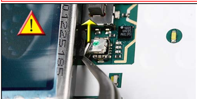
15. Very gently, open the COAX CONNECTOR by using angled tweezers.
