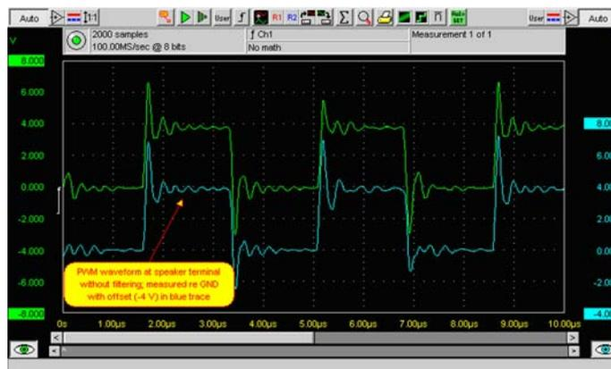
Figure 40 Differential output waveform of the Ext\_in\_IHF\_out out loop measurement when speaker is connected.
