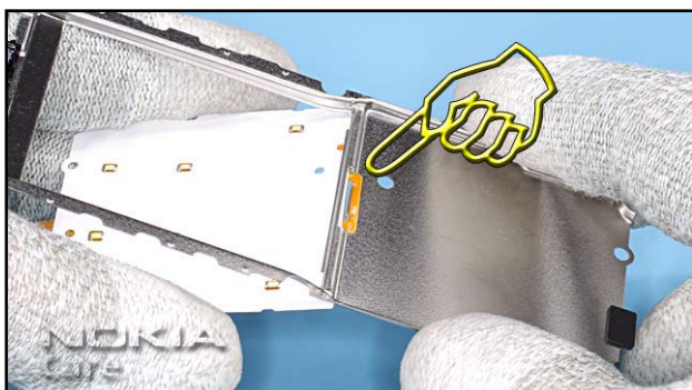
11. Separate the UI MODULE from the UI FRAME.
