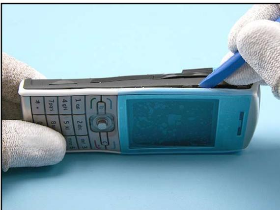
5. Slide the SS-93 along the edge to unlock the snaps.
