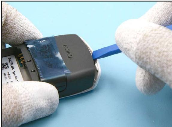
4. Unlock the A-COVER with the SS-93 starting on the top side of the phone.
