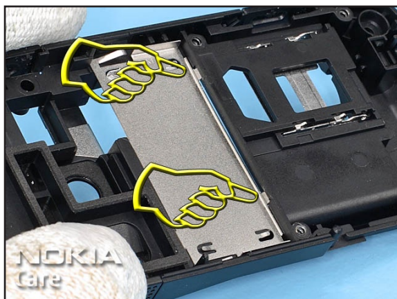
3. Secure the C-COVER METAL PLATE by pressing it into position.
