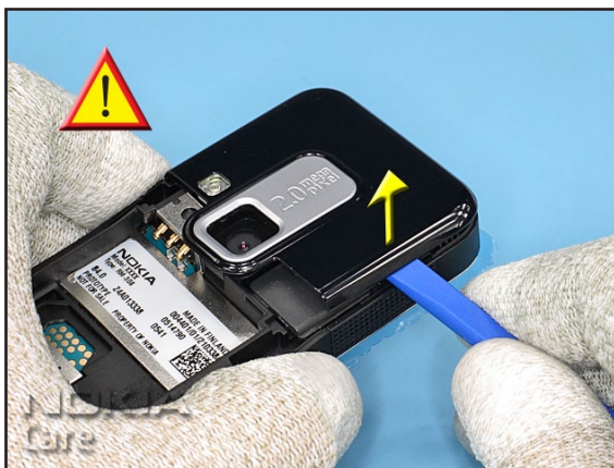
4. Place the SS-93 between the C-COVER and the ANTENNA COVER ASSY, and release the clips beginning on the shown side.
