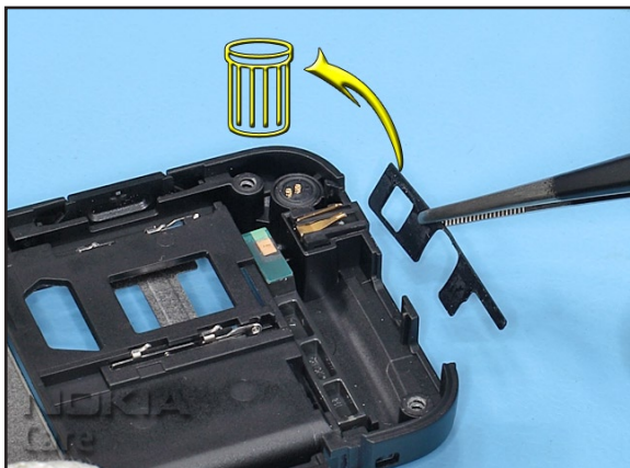
24. Remove the CONNECTOR LABEL and discard it.
