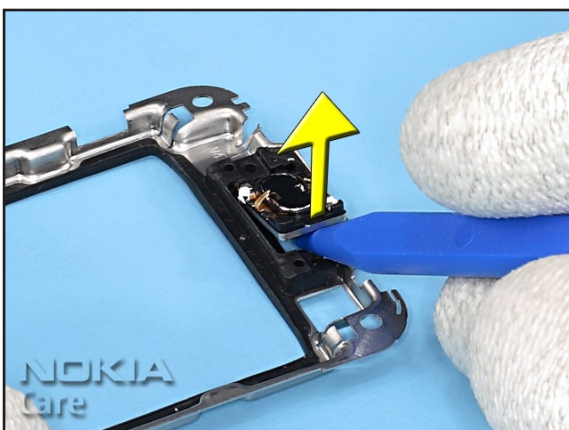
17. Lift the EARPIECE with the SS-93 and remove it.
