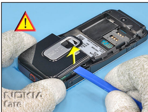
6. Release the last clip and remove the ANTENNA COVER ASSY.
