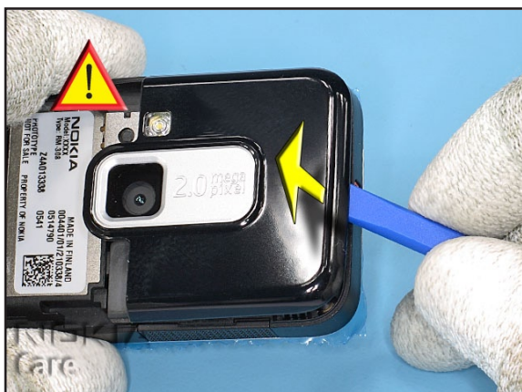
5. Release the clip on the top of the unit.
