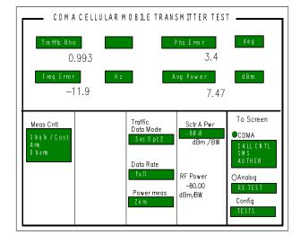
Simultaneous and transmitter tests is another feature of the HP 8924C. Simultaneous measure- ments results in much reduced test time. To make simultaneous receiver sensitivity and transmitter measurements:
