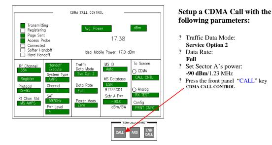
While service option 001 calls are useful for the verification of CDMA mobile functionality, parametric tests cannot be accurately made in this mode. The TIA IS-98A minimum performance standard recommends that testing be made using service option 002. In service option002, the mobile under test demodulates the rceived signal and then re-transmits this data to the HP 8924C. This mode allow accurate receiver performance measurements.
