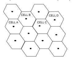
trum technology, all users share a range of the radio spectrum. CDMA cell coverage is dependent upon the way the network is designed. For each system 3 characteristics must be considered: coverage, quality, and capacity. These 3 must be balanced for desired lever of performance.
