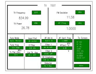
Test Mode Commands: CP Mode AMPS Load synthesizer to channel 300 Turn on carrier Set ATT power level from 1 to 7
