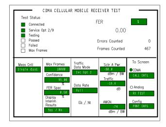
The other key receiver measurement for CDMA phones is the FER with AWGN test. In this test, large amounts of uncorrelated noise is added to simulate the actual conditions encountered by a CDMA phone in actual use. To make this measurement:
