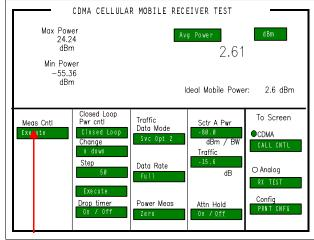
The ability to do min/max power measurements just by selecting Execute is another advanced feature of the HP 8924C. In this screen you can also control and test each power step while comparing Ideal Mobile Power to actual Avg Power measurements.
