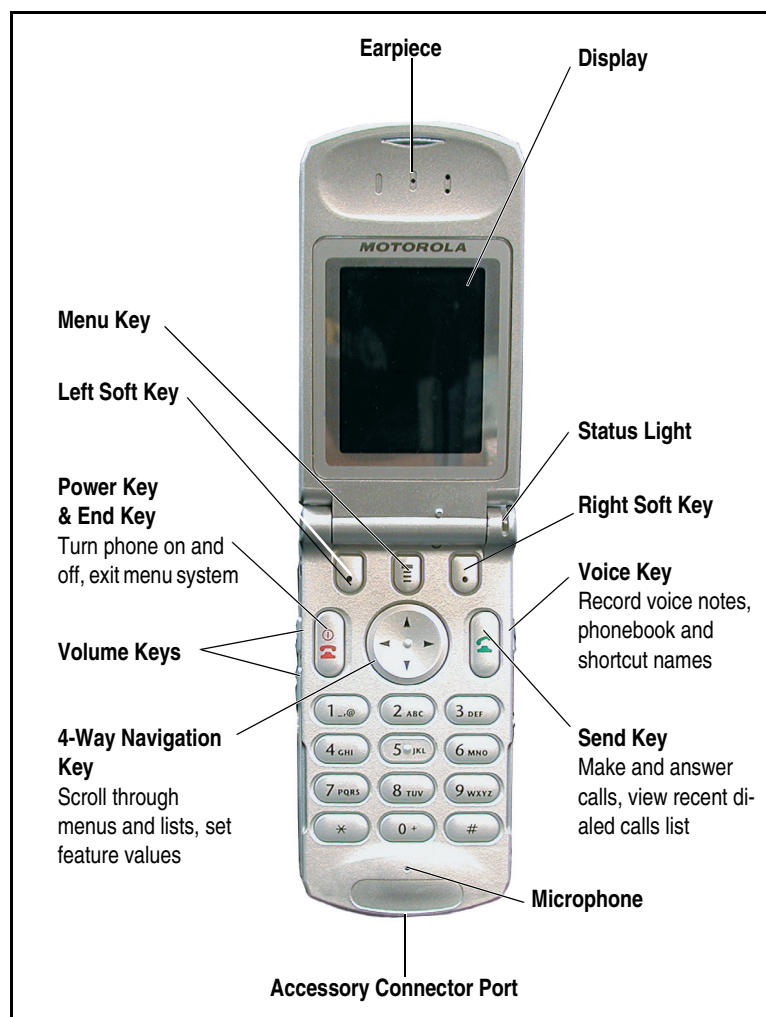
Figure 1. PF B65 Phone Controls, Indicators and I/O
