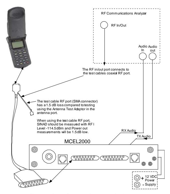
**Connections for Testing and Adjustments**
