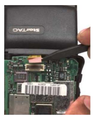
Step 2. With your thumbs, pry the side tabs away from the board assembly to allow it to be easily removed. Starting at the top of the board, lift the board assembly out of the front
