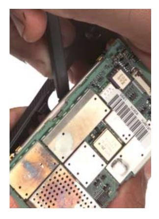
Step 3. Pull the tape off of the microphone connector and pull the connector out.
