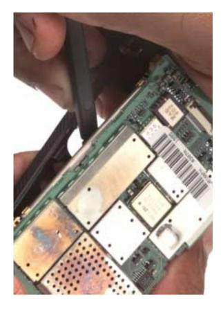
Step 3. Pull the tape off of the microphone connector and pull the connector out.
