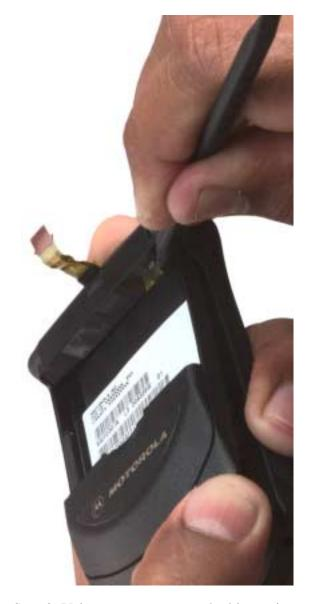
Step 2. Using tweezers, press the hinge pin button in and over toward the middle of the flip. Also, move the hinge pin section above the button toward the middle of the flip. Note: When reassembling the flip, the button will click back into place. Remove the flip by pulling up on the hinge pin side and out on the other side. The hinge shaft may come
