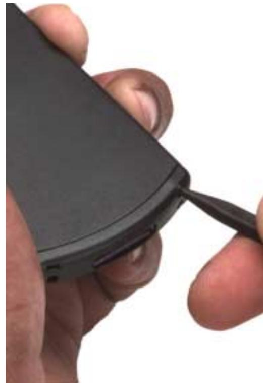
Step 2. Press and push corner outwards with left thumb while right hand twists phone like a rag.
