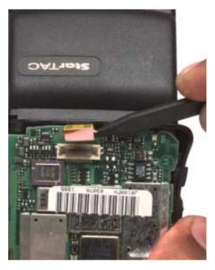
Step 2. With your thumbs, pry the side tabs away from the board assembly to allow it to be easily removed. Starting at the top of the board, lift the board assembly out of the front
