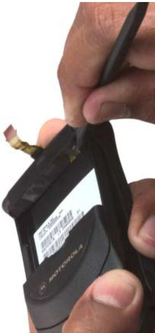
Step 2. Using tweezers, press the hinge pin button in and over toward the middle of the flip. Also, move the hinge pin section above the button toward the middle of the flip.
