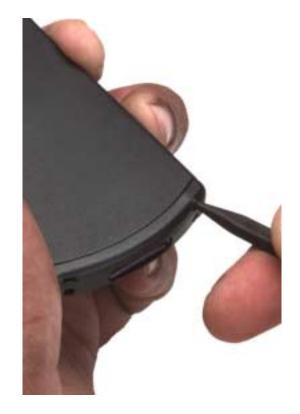
Step 2. Press and push corner outwards with left thumb while right hand twists phone like a rag.
