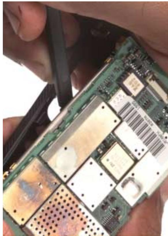
Step 3. Pull the tape off of the microphone connector and pull the connector out. Remove antenna tube.
