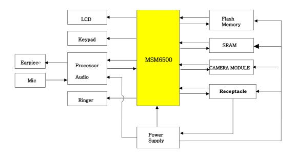
[Figure 2-2] Block Diagram of Digital/Voice Processing Part
