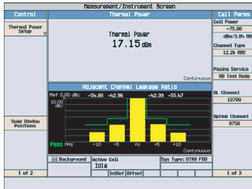
Fig. 4-33-5 Output Level at Isolator Input (IS200.3. In)
