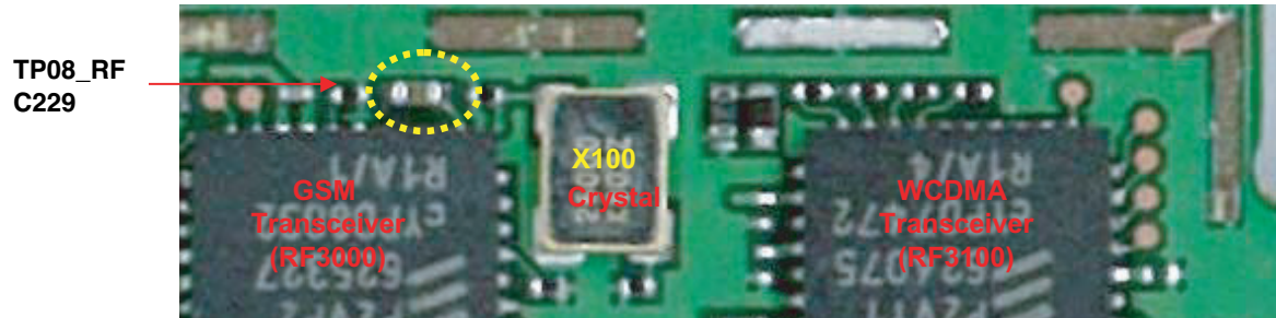
Figure 4-10-1. Test point (26MHz at TX part)
