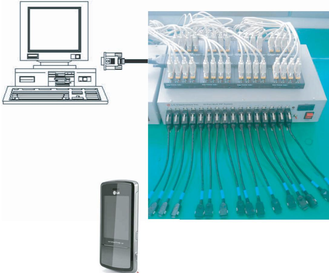
**Figure 6.1 describes download and upgrade setup on KF510**
