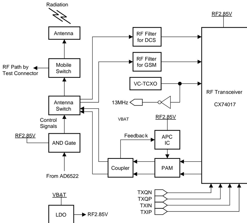
Figure 9-3. RF Blockdiagram.
