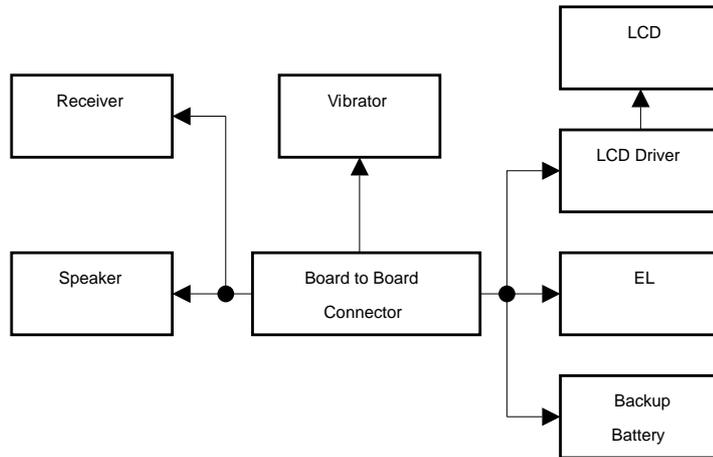
Figure 9-2. FPCB Blockdiagram.
