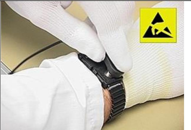
1. Make sure the ESD antistatic wrist strap connect to the ground is normal.
