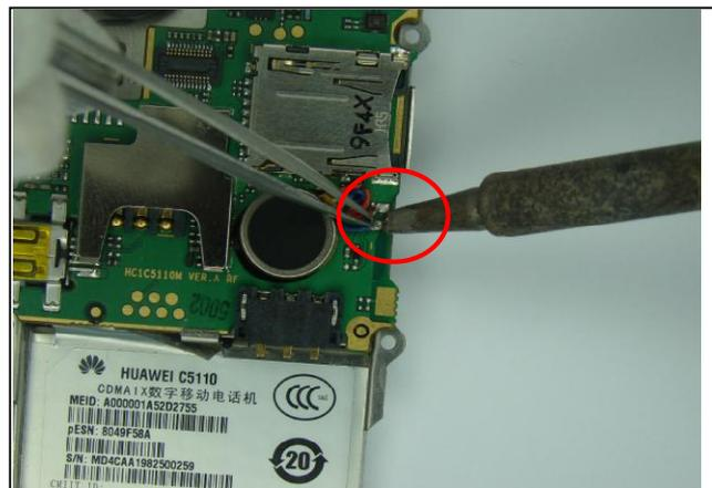
12. Solder motor onto main board and place it onto the location.
