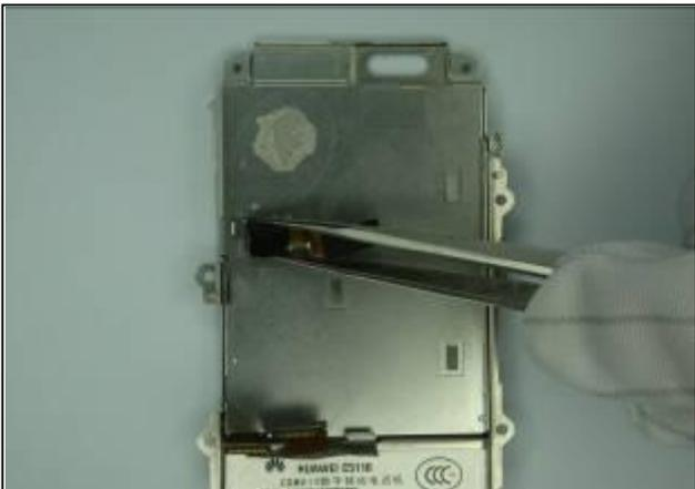
21. Camera is pasted onto the shield sheet, remove camera carefully.
