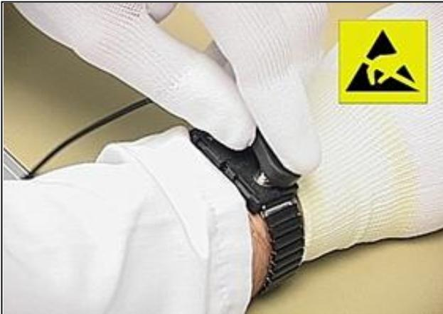
1. Make sure the ESD antistatic wrist strap connect to the ground is normal.
