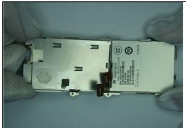
4. Place the shield sheet onto LCD.
