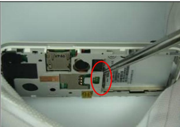
11. Loosen the lock according to the figure above.
