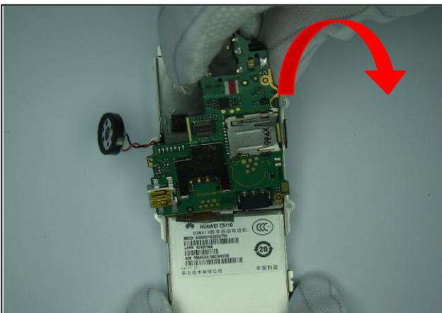
17. Turn the main board according the direction of arrowhead.
