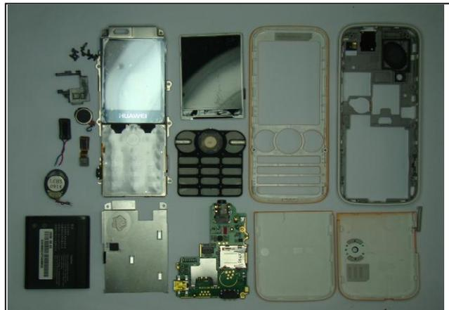
24. Disassembly process is completed.
