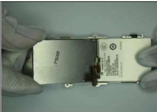
3. Place LCD onto the shield cover.
