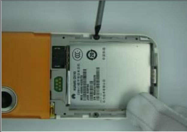
19. Screw on the two screws. If you use electrical screwdriver to fix screw, the torque is  $1.0 \pm 0.1$  kgf.cm.
