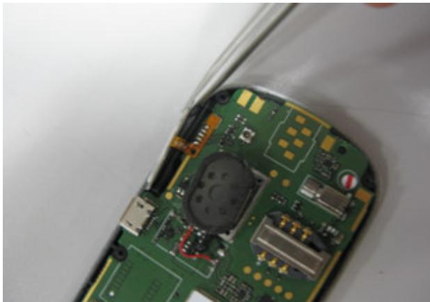
Step 5: Separate the Main PCBA from Furnished front casing
