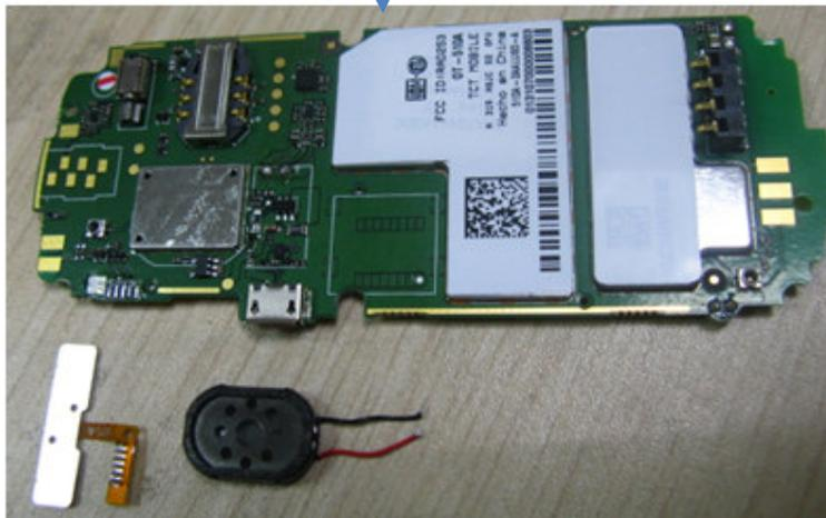
Step 9: Remove the following components from main PCBA with hot wind gun.
