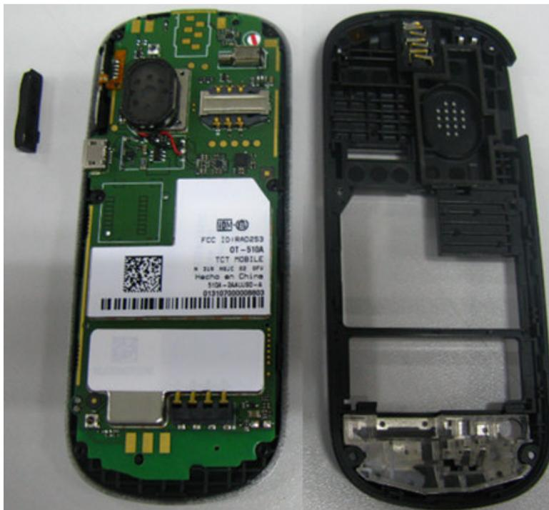
Step 3: Separate ANTENNA\_ASM and Audio Jack from Furnished Frame by tweezers
