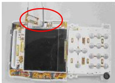
Use a tweezers to release the LCM connector (see the red circle) carefully.
