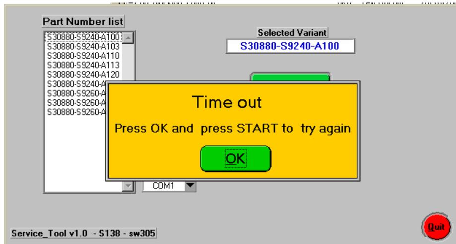
Press OK, remove the battery and serial connector and do the test again. If you meet the same problem
