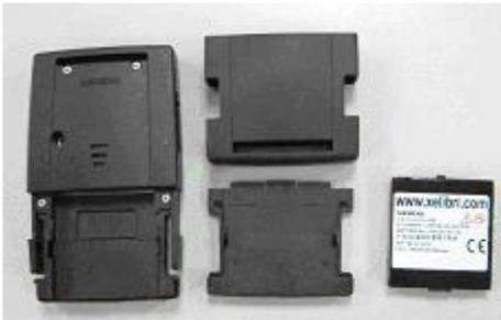
Remove the battery connector, clip cover and battery.
