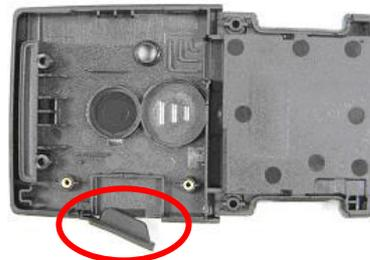
Assemble the I-O Door on the Back cover.
