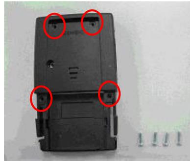
Remove the 4 screws (size 1,6 \* 7,5mm) on the back cover.
