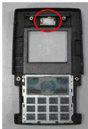
Take out the keypad from the front cover. (The spare part: front cover, contains a lens and sponge; Never remove the lens from the front cover.) Speaker on the front cover. (Do not remove speaker if not damaged)
