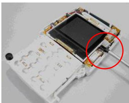
Open the LCM positioning tab (see the red circle) Push the LCM bracket positioning tab slowly and carefully. Use some strength upward
