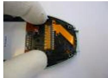
Clip the keypad assy around the microphone
